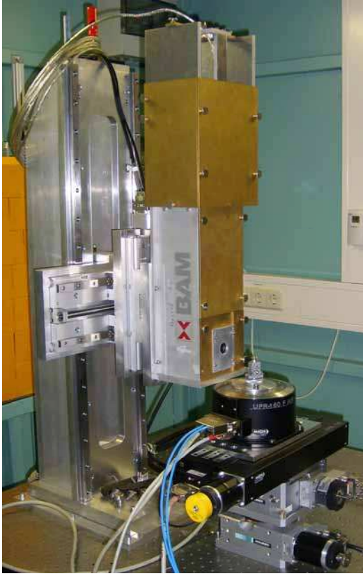
FIG. 6: (Color) Detector systems of the TopoTomo beamline mounted on xy-translation stages with a sample manipulator in front. Left: BAMline macroscope with pco.4000 CCD camera, right: OptiquePeter microscope with ESRF FReLoN 2k14bit [23, 67, 78].
