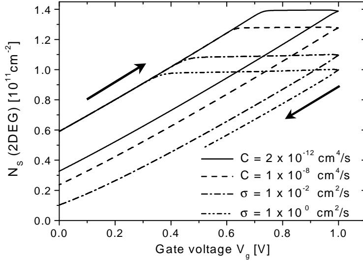
**Figure 5.** Calculated hysteresis in the  $N_s$ - $V_g$ -characteristic for the Auger process and for the phonon processes only. Different coefficients for the rate equation and a sweep duration of 1 hour are used.
