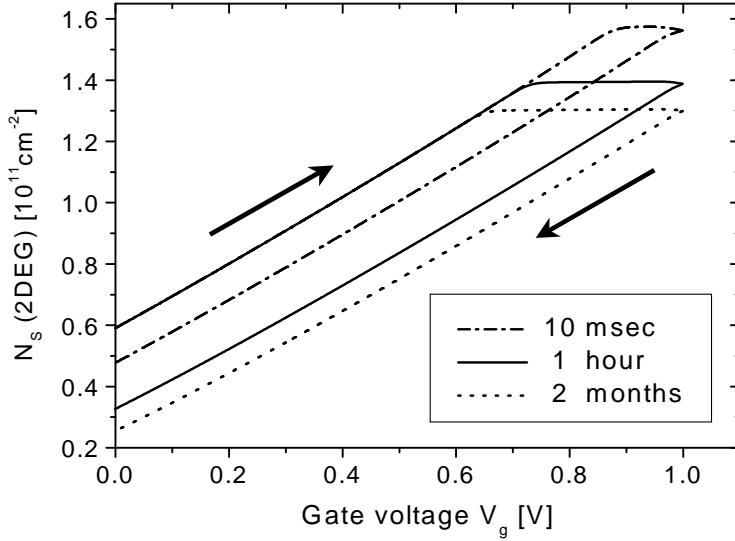
**Figure 4.** Hysteresis within the  $N_s$ - $V_g$ -characteristic calculated with different sweep durations and an Auger coefficient of  $C_{Auger} = 2 \times 10^{-12} m^4/s$  [5].
