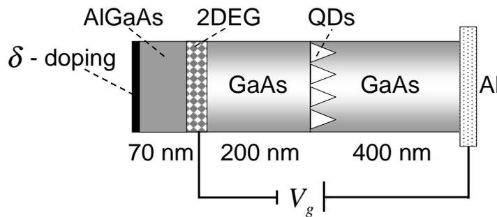
**Figure 1.** Sketch of the GaAs/n-AlGaAs field effect transistor with InAs QDs. The gate voltage  $V_g$  is applied between the two-dimensional electron gas and the Schottky contact (Al). The resulting conduction band edge is displayed in Fig. 3. The layers are (from left to right):  $10^{12}/\text{cm}^2$   $\delta$ -doping with Si; 70 nm  $\text{Al}_{0.25}\text{Ga}_{0.75}\text{As}$  barrier; 200 nm GaAs; 1.75 monolayer InAs (dots); 400 nm GaAs; 100 nm Al as top gate.
