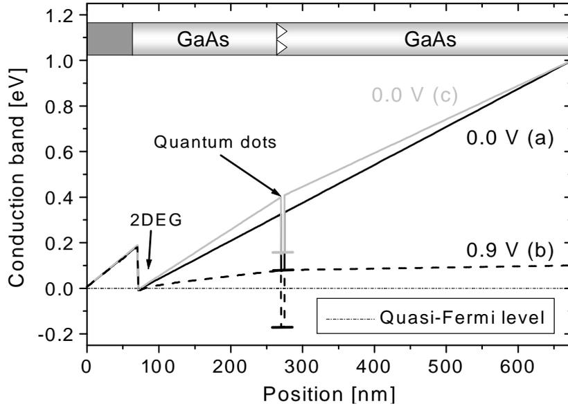
**Figure 3.** Calculated conduction band edges of the FET displayed in Fig. 1 for different gate voltages  $V_g$ . See Fig. 2 for the corresponding points within the hysteresis – indicated with (a), (b) and (c).
