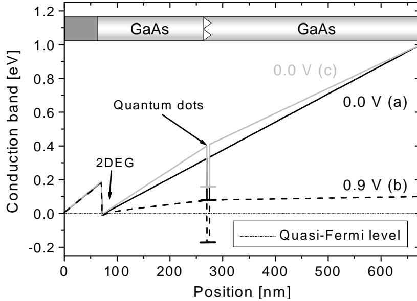
**Figure 3.** Calculated conduction band edges of the FET displayed in Fig. 1 for different gate voltages  $V_g$ . See Fig. 2 for the corresponding points within the hysteresis – indicated with (a), (b) and (c).
