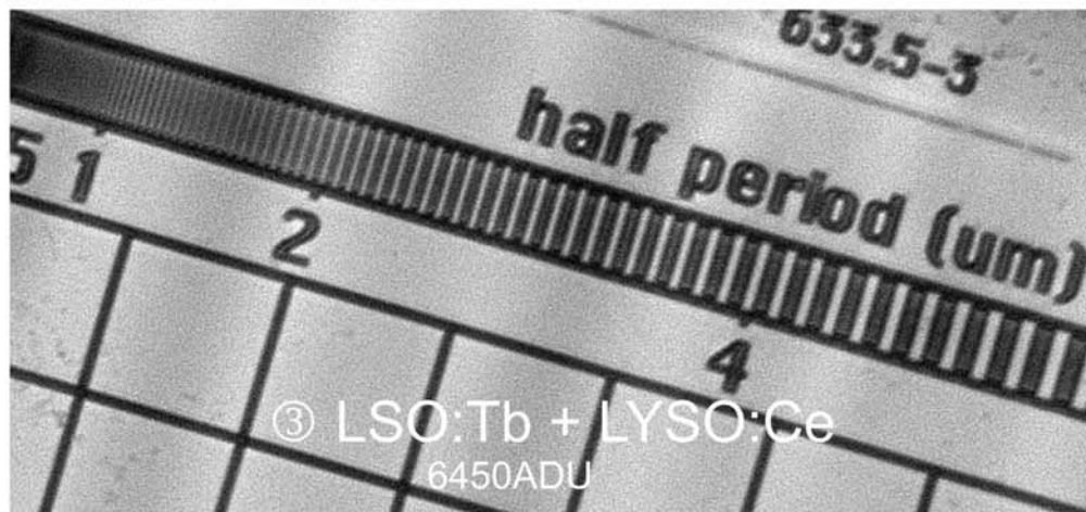
Demonstration of the spatial resolution achievable with a scintillator stack consisting of two layers (15x magnification / NA = 0.3 objective). The image 3 is a summation of image 1 and 2 detected by selecting the different emissions of the scintillator multi-layer via optical filtering. 161x168mm (300 x 300 DPI)
