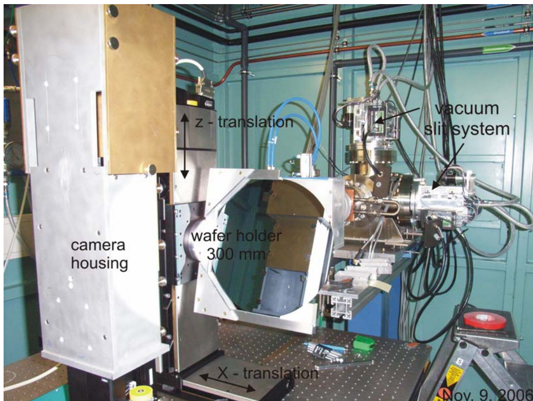
Fig.1: Experimental station of the digital white beam topography with commercial 300 mm Si - wafer
